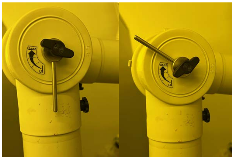
Figure 1 Evacuation switch schematic. Left depicts closed, and right depicts open.
